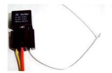
Terminal power lines: white connected relay 86 feet, 85 feet by 12 V dc battery positive, 87 feet series power supply circuit.
